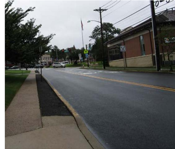
A rain garden can be installed in the turfgrass along the side of the church to capture, treat, and infiltrate stormwater runoff from the roof. An existing asphalt strip adjacent to the sidewalk can be replaced with a series of stormwater planters that could capture stormwater from the roadway. A preliminary soil assessment suggests that more soil testing would be required before determining the soil's suitability for green infrastructure.
