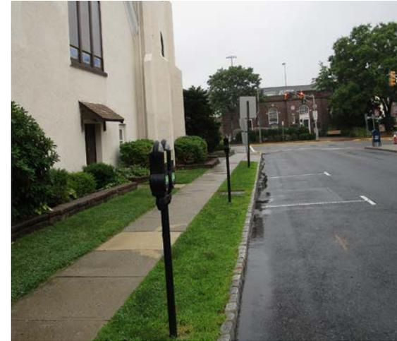
A rain garden can be installed in the turfgrass and shrub area along the side of the building to capture, treat, and infiltrate stormwater runoff from the roof. Parking spaces in the parking lot can be converted to porous pavement to capture and infiltrate stormwater runoff from the front parking lot. A preliminary soil assessment suggests that more soil testing would be required before determining the soil's suitability for green infrastructure.
