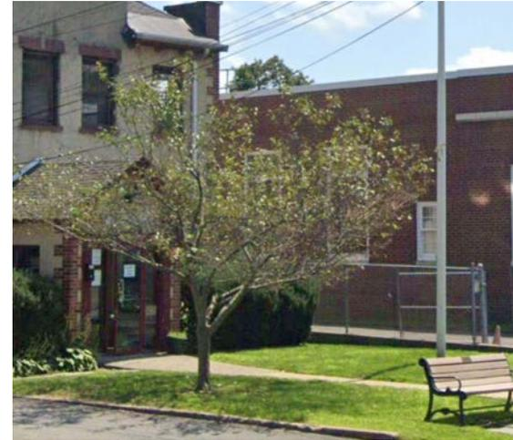
A rain garden can be installed at the front of the building around the flag pole by disconnecting the downspout from the corner of the building into the garden. A preliminary soil assessment suggests that the soils have suitable drainage characteristics for green infrastructure.
