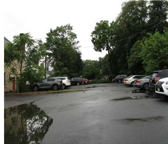
Parking spaces in the parking lot at the back of the building can be converted to porous pavement to capture and infiltrate stormwater runoff from the parking lot. Porous pavement can also help drain the large pooling area of the parking lot. A preliminary soil assessment suggests that the soils have suitable drainage characteristics for green infrastructure.
